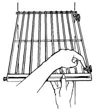
**1.** While pressing tabs on shelf supports on right wall, lift shelf out of grooves in supports.
